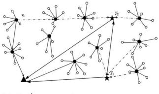
▲ Sink node ★ Heterogeneous node ● Cluster head node ○ Ordinary node
