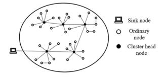
Figure 2: Structural diagram of heterogeneous sensor networks
