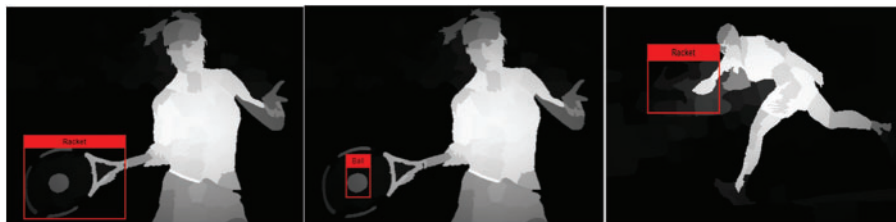
Figure 6: Similar-pixels clustering for object detection
