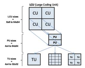
Figure 1: Coding structure in HEVC standard
