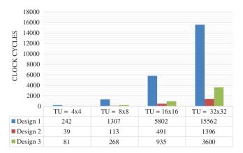
Figure 7: Number of clock cycles to reconstruct 4/8/16/32 residual block
