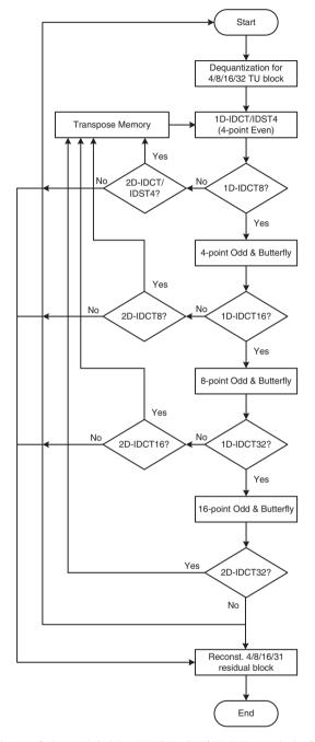
Figure 3: Dataflow of the HLS 2D-DE/IDCT/IDST module for HEVC decoder
