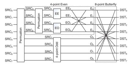
Figure 2: Flowchart of 8-points 1D-IDCT based on chen's algorithm
