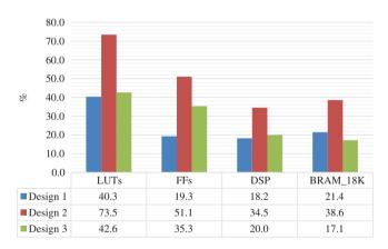
Figure 6: HLS synthesis results of HEVC 2D-DE/IDCT/IDST module
