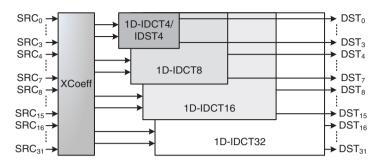
Figure 10: 1D-IDCT/IDST hardware architecture
