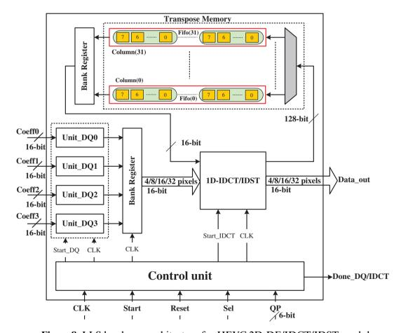
Figure 8: LLS hardware architecture for HEVC 2D-DE/IDCT/IDST module
