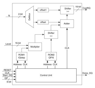
Figure 9: Hardware architecture of Unit DQ
