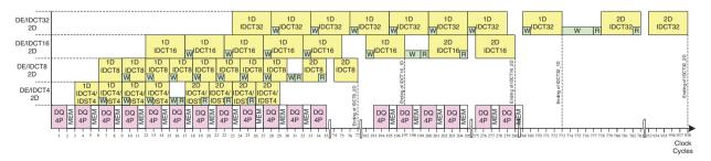
Figure 11: Timing diagram for HEVC 2D-DE/IDCT/IDST module
