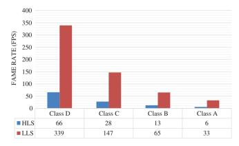
Figure 12: Frame rate comparison between HLS and LLS designs for A, B, C and D video class
