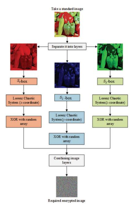
Figure 1: Design of proposed encryption scheme
