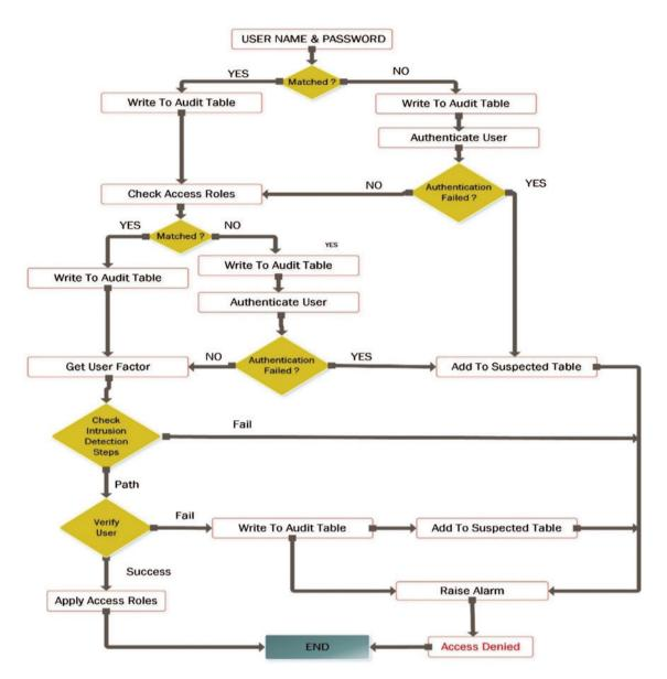
Figure 6: Overall access steps with intrusion detection
