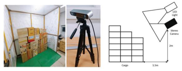
Figure 7: Verification environment configuration
