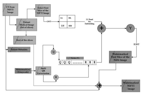
Figure 2: Block diagram of hybrid method for digital watermarking process
