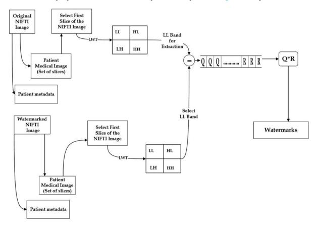
Figure 3: Block diagram of hybrid method for watermark extraction
