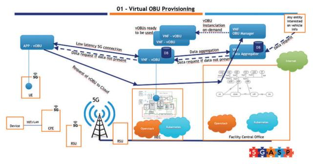
Figure 4: Virtual On-Board Unit (vOBU) NetApp
