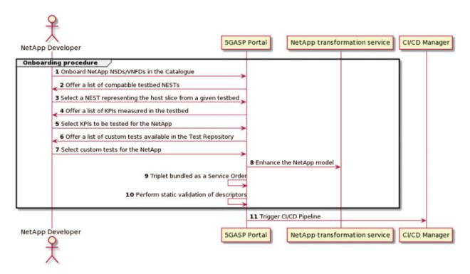
Figure 3: NetApp onboarding and connection to CI/CD service
