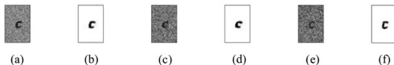
Figure 7: Output of SDAE for different percentage of noise levels: (a) Image with 20% noise variance (b) Output of SDAE at 20% noise (c) Image with 40% noise variance (d) Output of SDAE at 40% noise (e) Image with 60% noise variance (f) Output of SDAE at 60% noise
