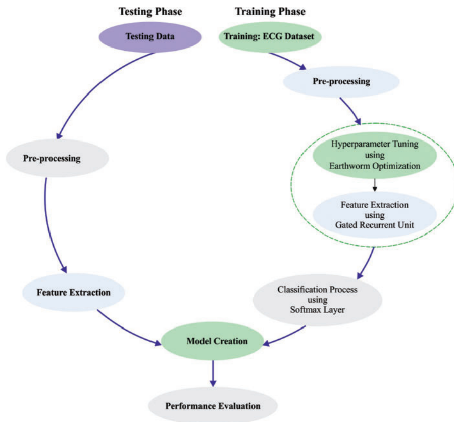
Figure 1: Overall process of IBECG-SP method
