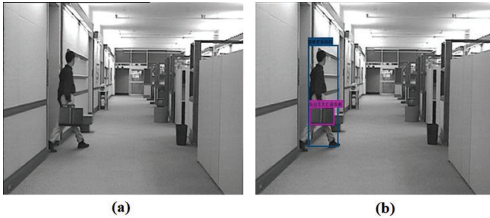
Figure 7: Visualization analysis results of EODM-AAS model on hall monitor dataset (a) Original image, (b) Output image
