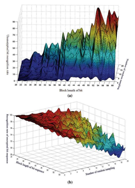
Figure 3: Encryption performance test. (a) Test results without file, (b) Encrypted file detection results
