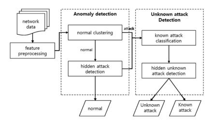
Figure 1: Processes of the proposed hybrid intrusion detection
