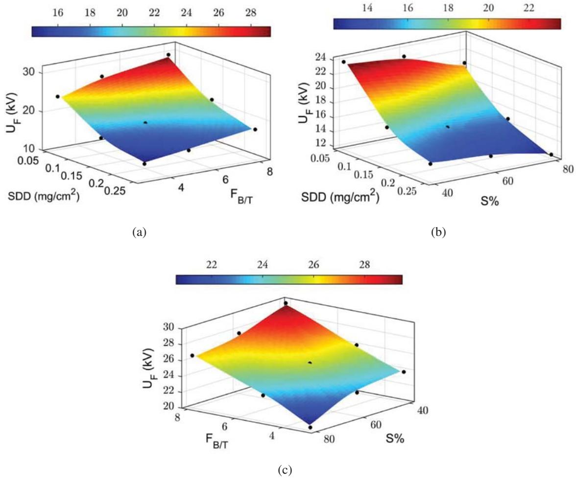
**Figure 9:** (a) The flashover voltage of scenario D (a) SDD and S under  $F_{B/T} = 3$ . (b) SDD and  $F_{B/T}$  under  $S = 40\%$ . (c)  $F_{B/T}$  and S under  $SDD = 0.15 \text{ mg}/\text{cm}^2$
