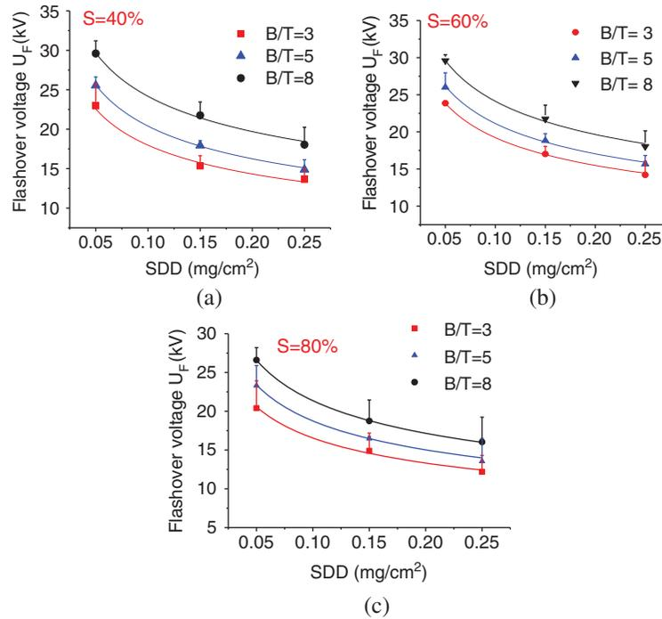
**Figure 8:** UF-SDD curve. (a)  $S = 40\%$ ; (b)  $S = 60\%$ ; (c)  $S = 80\%$
