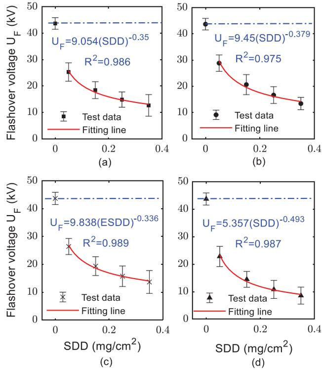
**Figure 3:** Flashover voltage of insulator under different modes and relative humidity of 75%: (a) Scenario A; (b) Scenario B; (c) Scenario C; (d) Scenario D
