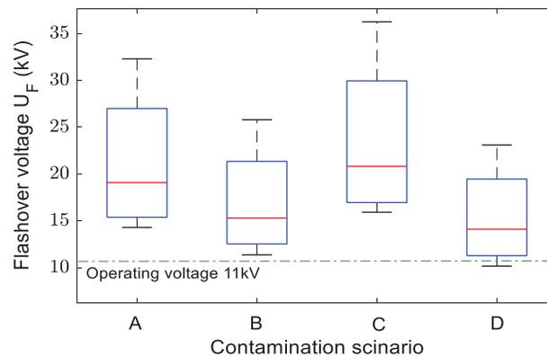
**Figure 6:** FOV of the proposed scenarios under RH of 75% and SDD from 0.05–0.35 mg/cm<sup>2</sup>
