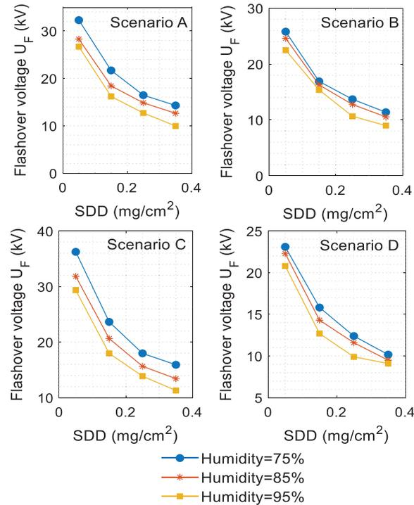
**Figure 7:** Flashover voltage of insulator for the proposed scenarios under different humidity
