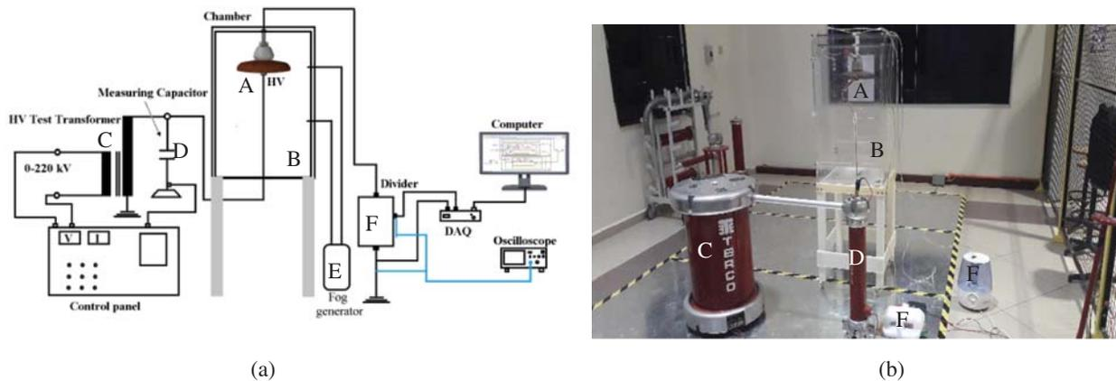
**Figure 2:** (a) Experimental setup circuit (b) laboratory test: A: the tested samples, B: chamber, C: transformer, D: capacitor, E: fog generator and F: control panel
