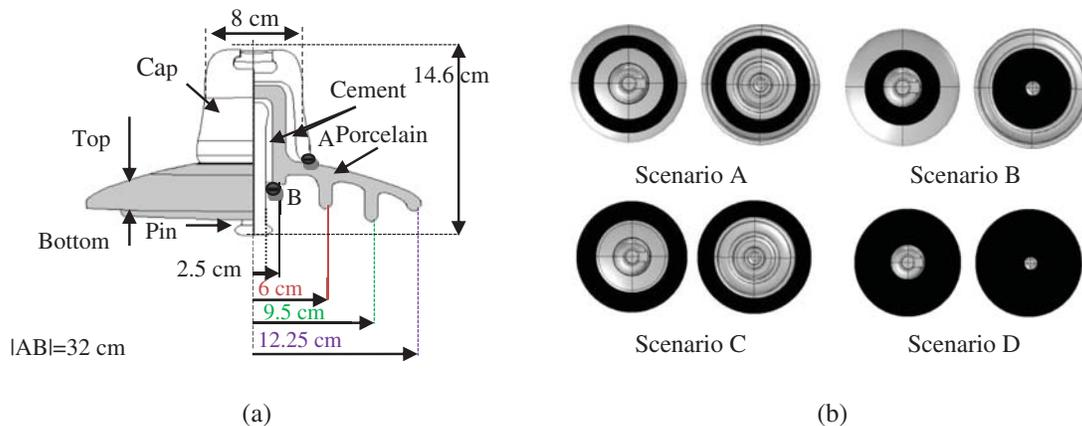
Figure 1: (a) Schematic of the insulator model; (b) Pollution distribution proposed scenarios
