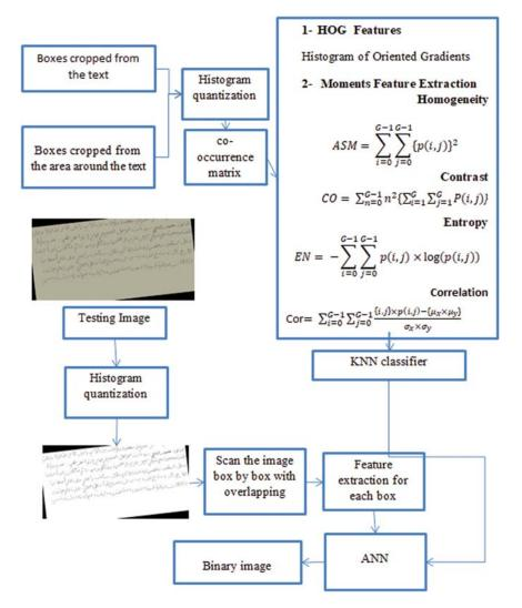
Figure 5: Framework of binarization step
