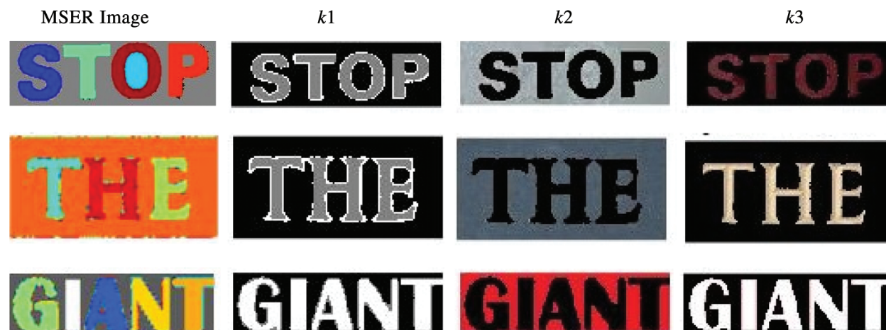
Figure 4: Separating foreground from background using K-means applied on the MSER images, where k = 3 is settled for obtaining clusters
