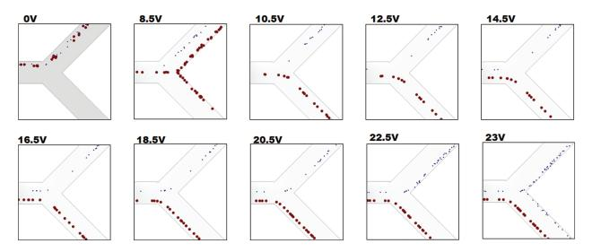
**Figure 8:** Simulation output shows the selective separation of Platelets (red) from *E. coli* (blue) when applied near-field potential using near filed electrodes. 8.5 V to 22.5 V found to be a range of voltages for platelet separation. After 23 V the *E. coli* transferred to platelet outlet
