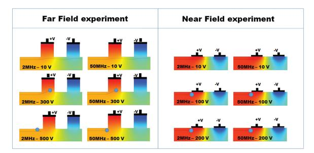
Figure S2: Particle trajectory when operated at above 2 MHz to 50 MHz show an adhering effect to the electrode when operated at high voltages whereas at low voltages particle flow through the its normal streamline
