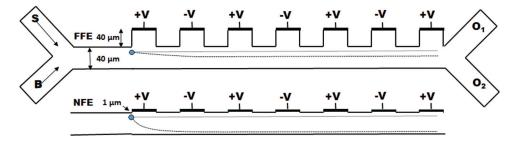
**Figure 2:** Schematic of the microfluidic channel represent placement of electrode for far filed (away from the channel) and near field (near to the channel) configurations and also exhibit the effect of electrode placement on distinct deflection (represented by the curved dotted line) of the particle from its streamline when operated at a fixed voltage
