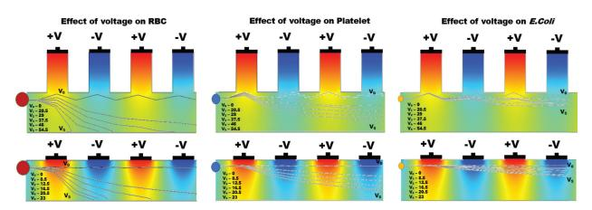
Figure 6: Simulation results show the effect of differential operating voltage from 0 to 55 V for far-field and 0 to 23 V for near field electrode placement applied on various particles (RBC, Platelets and *E. coli*) and the individual particle trajectories inside the active electric field region of the microchannel
