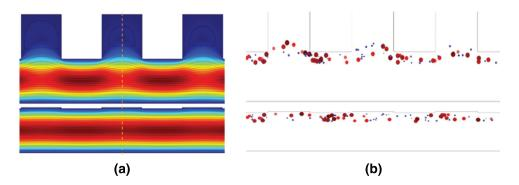
Figure 5: (a) The velocity distribution in the channel (b) particle movement for both far field and near field electrode placement
