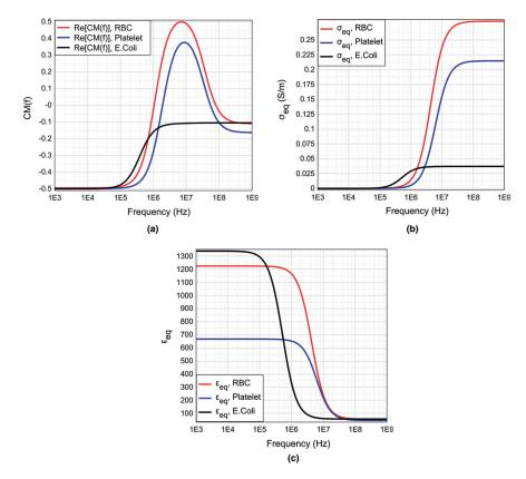
Figure 1: (a) The real part of CM factor, (b) equivalent electrical conductivity, (c) equivalent relative permitivity for RBC, Platelets and *E. coli* suspended in a medium obtained by using MyDEP [39] software. The CM factor for *E. coli* show a sigmoidal relation over the broad range of frequency 1 KHz to 1 GHz
