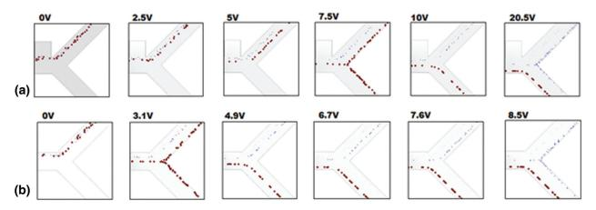
**Figure 3:** Simulation output for the selective separation of RBC (red) from Platelet and *E. coli* (blue) when applied far-field and near-field electrodes validate the simulation design parameters. Critical separation of RBC achieved at 7.5 V for far-field electrode position (first column) and the same for near-field electrode placement achieved at 3.1 V
