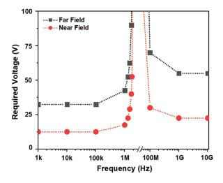
Figure 9: The simulation response obtained for an applied voltage for a change in operating frequency show a transition between 100 kHz to 1 GHz for a predefined particle trace
