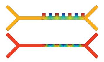
Figure S1: The simulation response for electrical field distribution when operated at 10 V (100 kHz)
