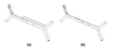
Figure 7: 3D model simulated using COMSOL Multiphysics show the separation of particles (RBC, Platelets and *E. coli*) when subjected to a non-uniform electrical field at an electrical potential of 12.5 V and 7.5 V in (a) Farfield electrode setup and (b) Nearfield electrode setup respectively
