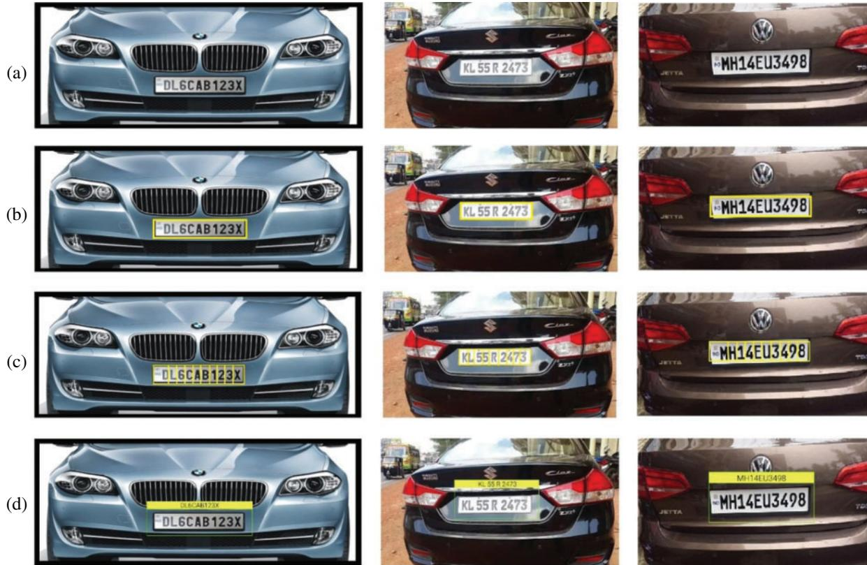
Figure 5: (a) Original images (b) LP detection images (c) Segmented images (d) Recognized images
