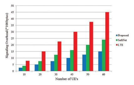
Figure 4: Overhead for signaling messages
