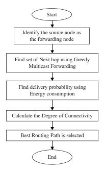
Figure 3: Flowchart for the routing process
