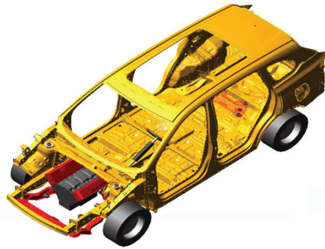
Figure 2: Rigid-flexible coupling model of the whole vehicle
