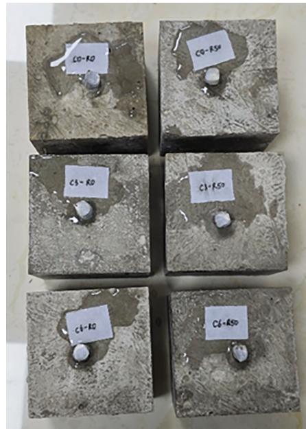
Figure 1: Photograph of the reinforced concrete specimen.
