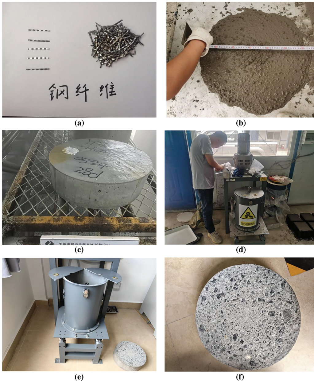
Figure 1: Testing process of SCC. (a) Steel fiber (Length: 0.18~0.22 mm); (b) After blending slump-flow test; (c) Standard curing of specimens; (d) Abrasion resistance testing machine; (e) Abrasion resistance test; (f) Test specimen of abrasion resistance
