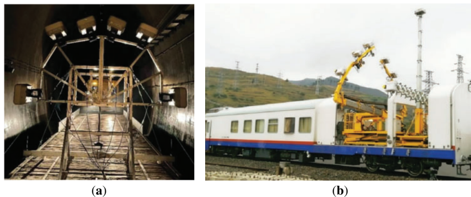
Figure 1: HSR tunnel inspection equipment configurations: (a) Vehicle-mounted A-CGPR antenna group (300 MHz) operating at standoff distances of 2.5–4 m; (b) High-speed rail tunnel inspection vehicle equipped with near-surface G-CGPR system (TR400/900 MHz combination antenna)
