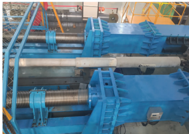
Figure 7: Mechanical properties test of decommissioned viscous dampers
