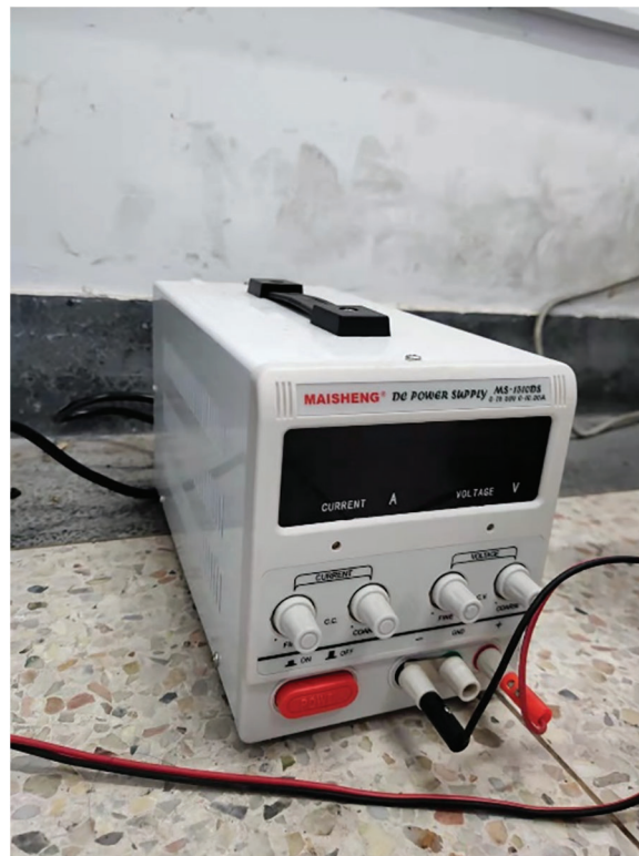
Figure 4: DC voltage stabilizing power supply
