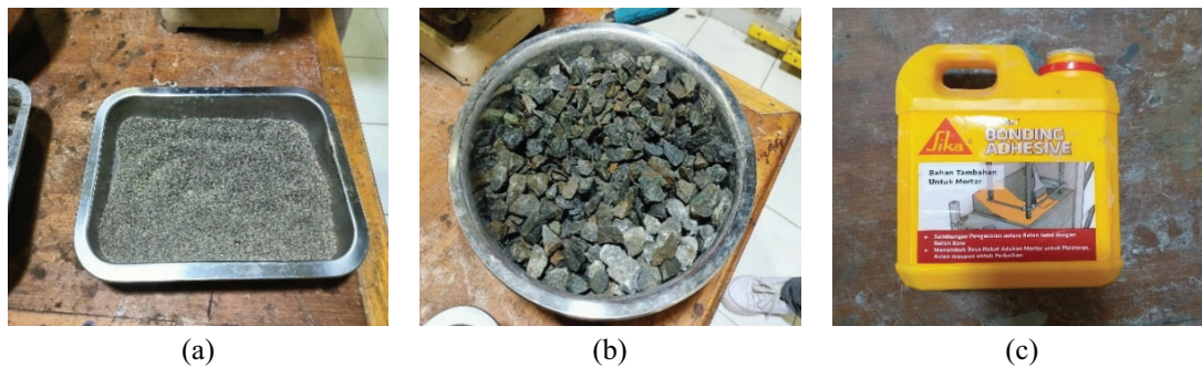
Figure 1: (a) Fine aggregate (b) Coarse aggregate, and (c) Bonding adhesive
