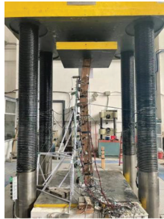
(c) C-2250-10-1: Buckling failure
