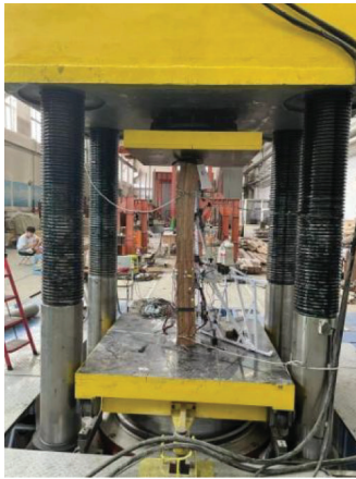
(b) C-1600-14-1: Both cracking failure of adhesive layers and buckling failure
