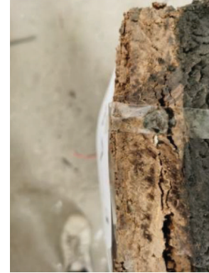
(a) C-850-14-1: Both cracking failure of adhesive layers and fibre tearing failure
