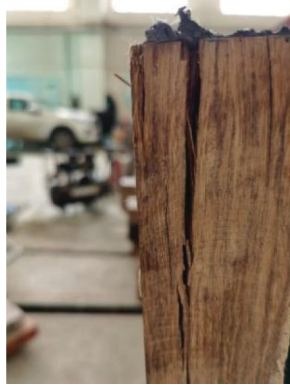
(a) C-850-14-1: Both cracking failure of adhesive layers and fibre tearing failure
