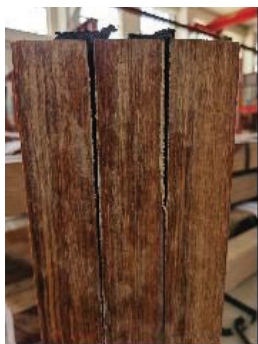
(a) C-850-0-1: Only cracking failure of adhesive layers
