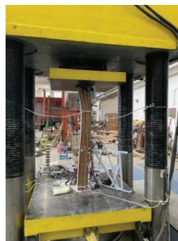
(b) C-1600-0-1: Both cracking failure of adhesive layers and buckling failure
