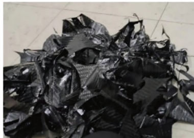
Figure 1: Original recycled CFRP prepreg scraps from CFRP product manufacturing factory
