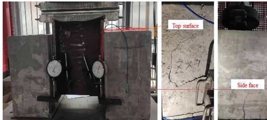
(a) PBL specimen with straight penetrating rebar
