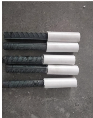
Figure 6: Physical diagram of the defect simulation
