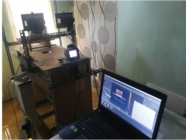
Figure 5: Testing concrete surface temperature used thermography and thermocouple method
