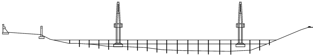
Figure 7b: Construction of main tower and girder 0#
