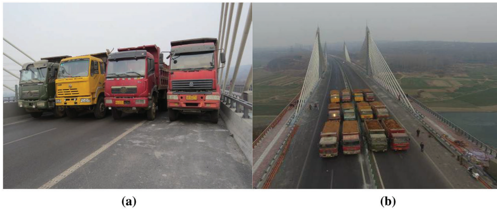
Figure 11: Photos of static load test
