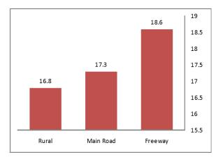
Figure 5a: Average SHM score of decks in single span bridges.
