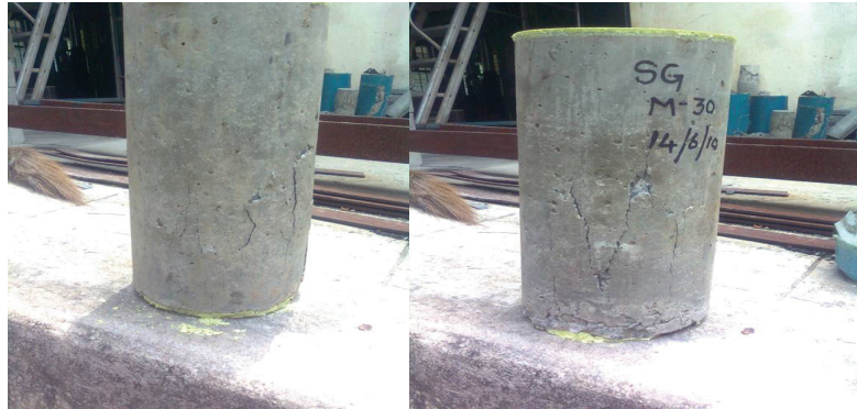
Figure 5: 1) Control specimen (Lateral Shear); 2) Control specimen (Cone Failure)
