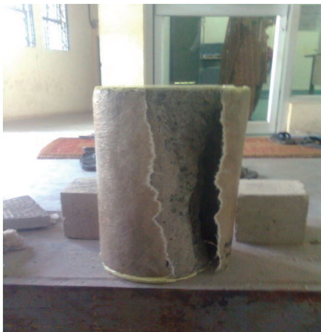
Figure 10: Failure Pattern in CSM
