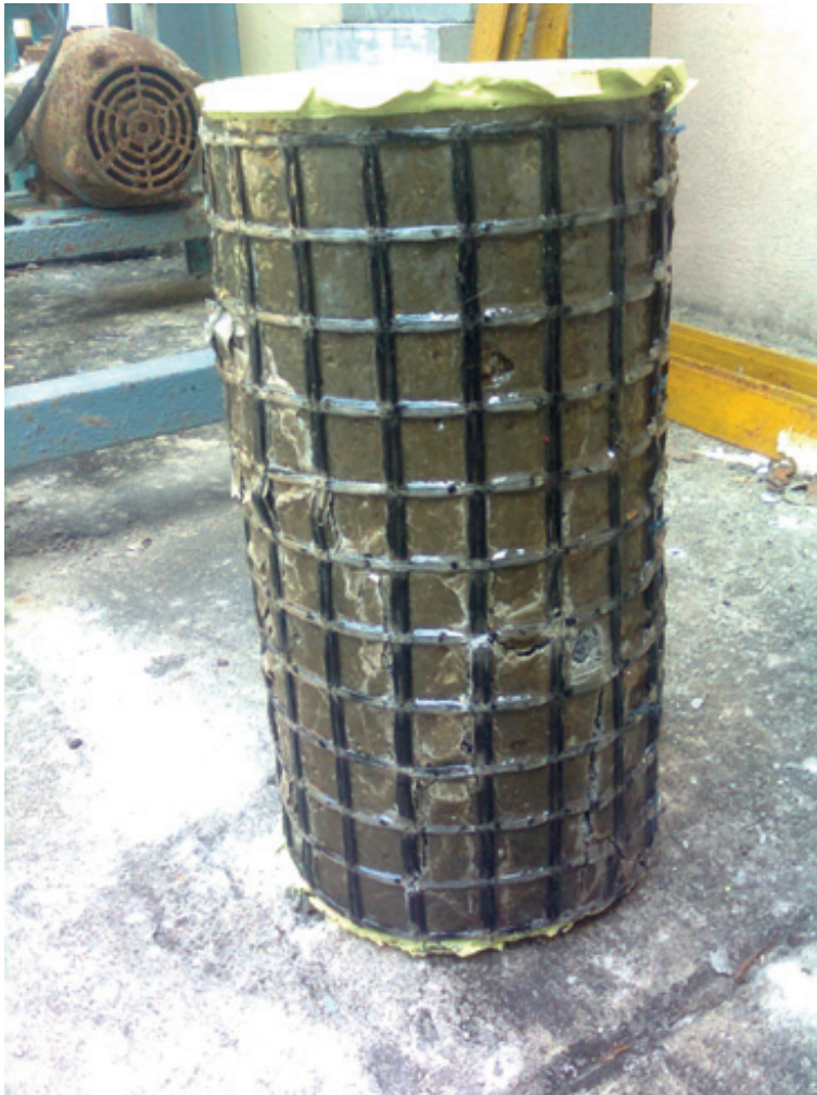
Figure 12: Compression failure of specimen confined with textile reinforcement
