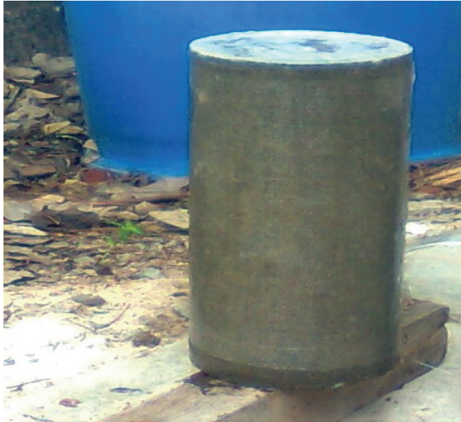
Figure 4: Specimen with its surface prepared
