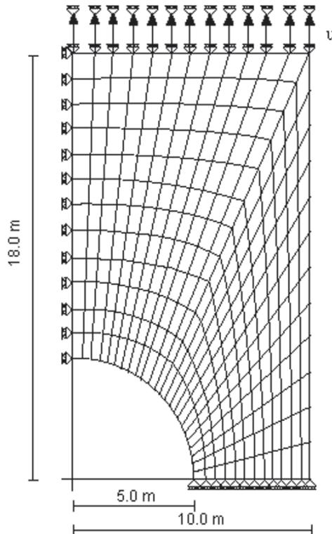
Figure 1: Perforated strip: geometry of the problem and finite element mesh.
