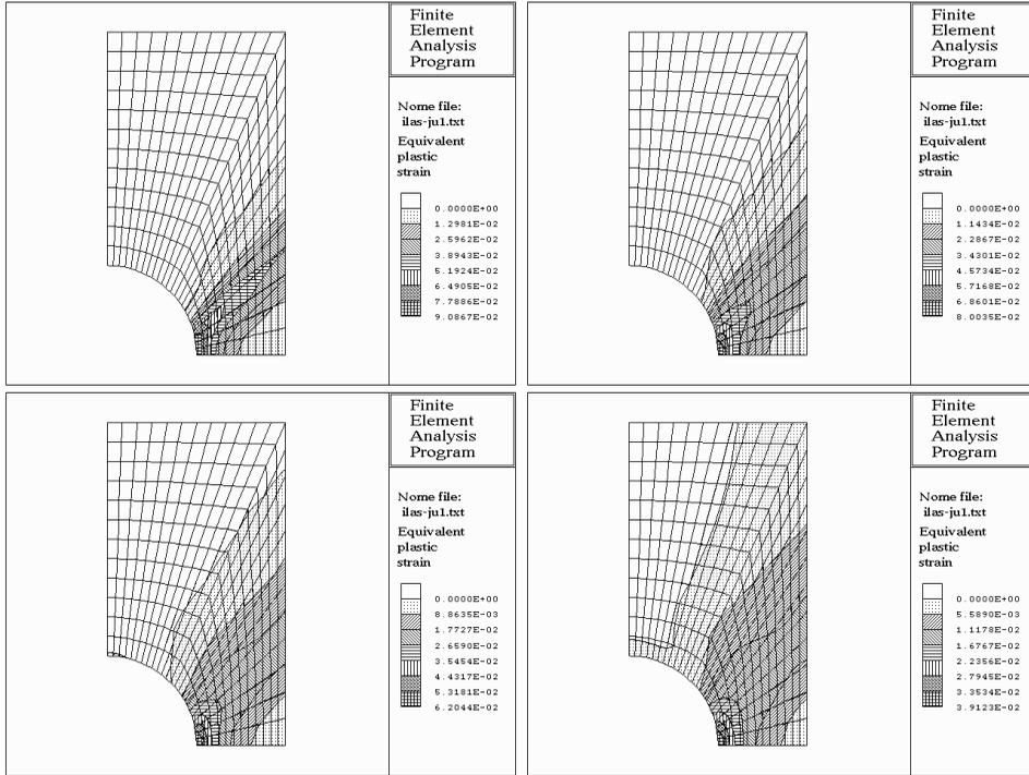
Figure 5: Contour plots of the equivalent viscoplastic strain in the strip for the final prescribed displacement  $u = 20 \text{ cm}$  and for increasing values of the prescribed loading rate. Top left:  $\tau = 0$  (rate-independent behavior). Top right:  $\tau = 0.1$ . Bottom left:  $\tau = 0.3$ . Bottom right:  $\tau = 1$ .
