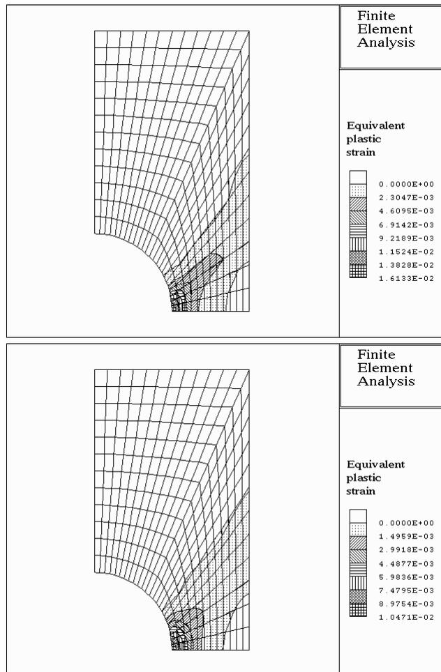
Figure 4: Contour plots of the equivalent plastic strain for the same prescribed displacement  $u = 6 \text{ cm}$  and with different prescribed loading rates. Top:  $\tau = 0$  (rate-independent behavior). Bottom:  $\tau = 0.1$  (prescribed loading rate).
