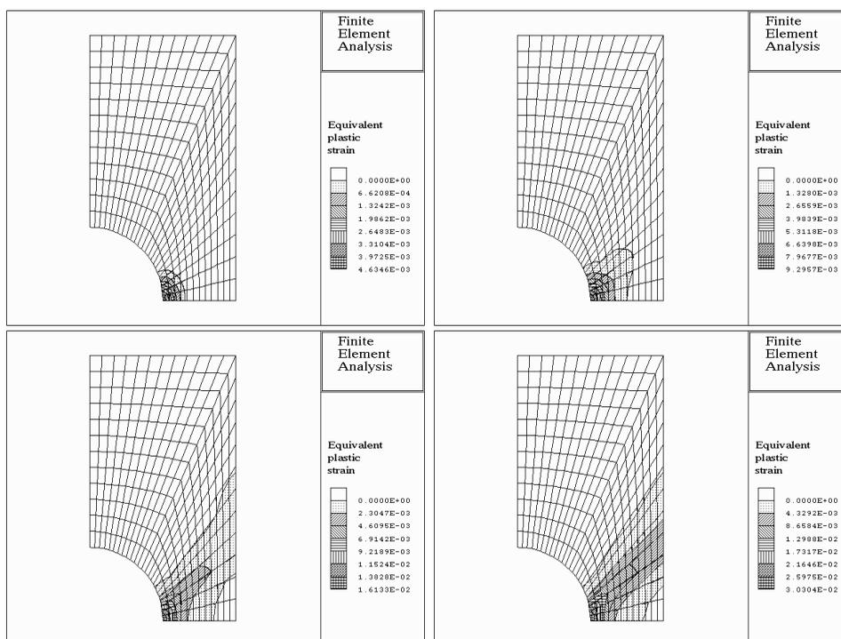
Figure 2: Evolution of the plastic process for an increasing upper edge prescribed displacement  $u$  and a rate-independent behavior. (Top left:  $u = 4$  cm. Top right:  $u = 5$  cm. Bottom left:  $u = 6$  cm. Bottom right:  $u = 8$  cm.)
