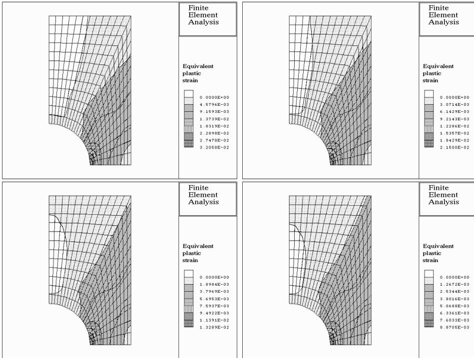
Figure 6: Contour plots of the equivalent viscoplastic strain in the strip for the final prescribed displacement  $u = 20 \text{ cm}$  and for increasing values of the prescribed loading rate. Top left:  $\tau = 1.5$ . Top right:  $\tau = 3$ . Bottom left:  $\tau = 6$ . Bottom right:  $\tau = 10$ .
