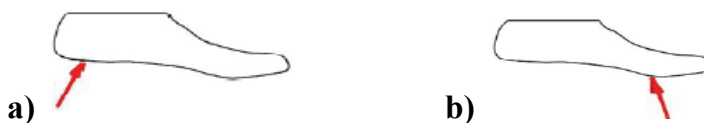
Figure 4: Schematization of the stance for the normal walk and related interpretation of the ISO 10328 standard: a) heel contact and b) toe-off
