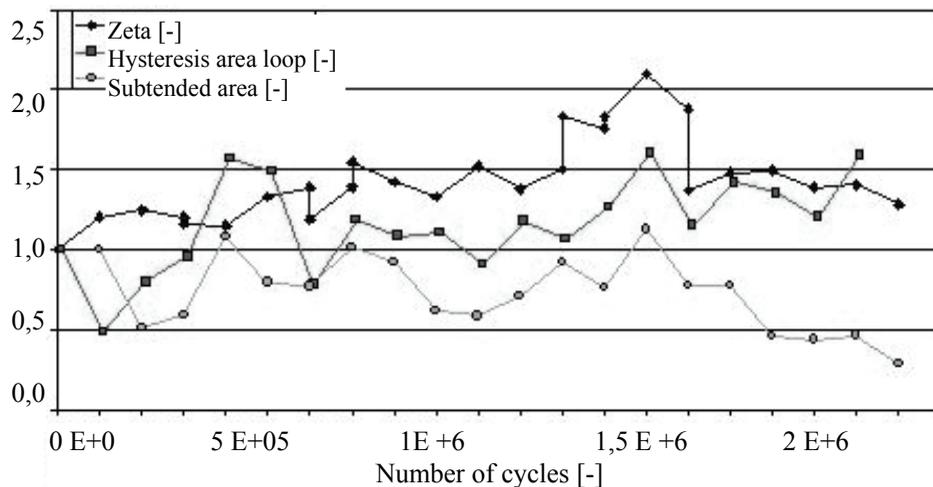
Figure 6: Modal damping, hysteresis loop area and subtended area by thermal profile variations during fatigue tests (C45\_1 steel specimen)
