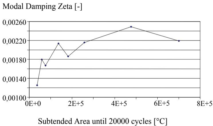
Figure 8: Subtended area up to 20000 cycles by thermographic acquisition vs modal damping (C40\_1 steel specimen)
