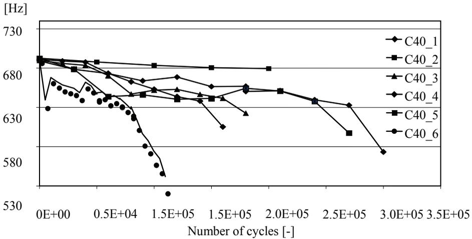
Figure 2: Resonance frequency variation during fatigue tests (C40 steel specimens)
