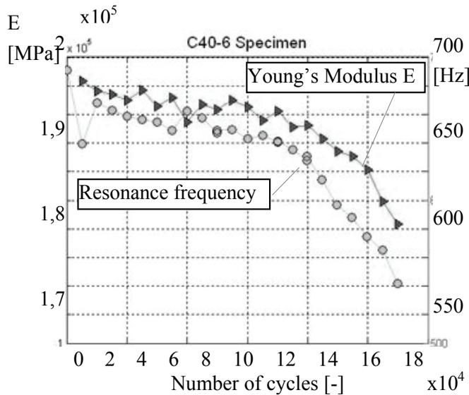
Figure 4: Resonance frequency and Young modulus variation during fatigue tests (C40\_6 steel specimens)
