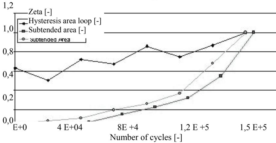
Figure 7: Modal damping, hysteresis loop area and subtended area by thermal profile variations during fatigue tests (C40\_1 steel specimen)
