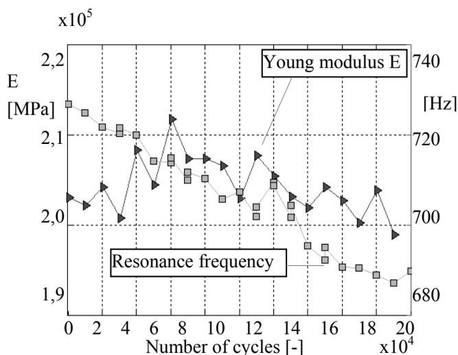
Figure 5: Resonance frequency and Young modulus variation during fatigue tests (C45\_1 steel specimens)
