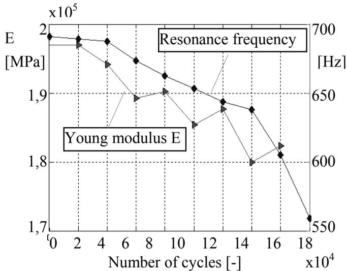
Figure 3: Resonance frequency and Young modulus E variation during fatigue tests (C40\_1 steel specimens)
