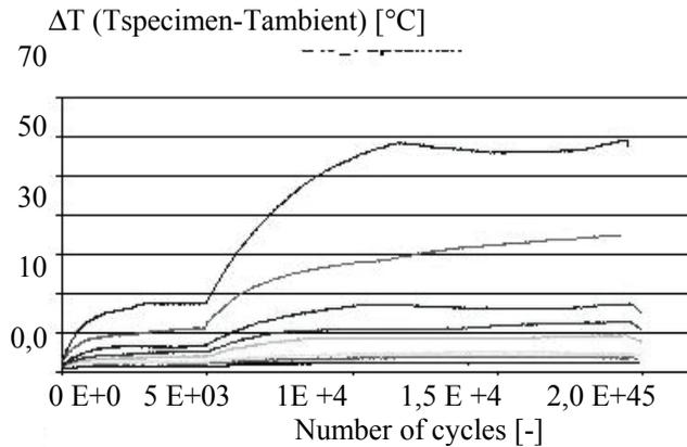
Figure 9: Thermal profiles (C40\_1 steel specimen)
