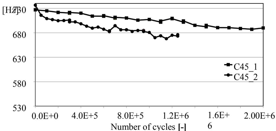
Figure 1: Resonance frequency variation during fatigue tests (C45 steel specimens)
