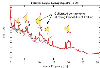
Figure 3: Potential Fatigue Damage Spectrum
