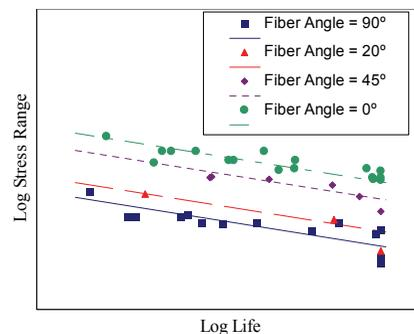
Figure 5: Fatigue Strength with Fiber Alignment
