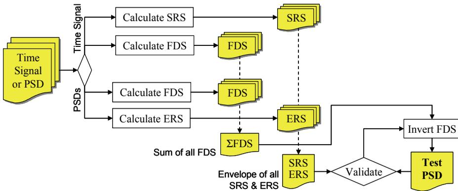
Figure 6: Mission Profile and Test Synthesis
