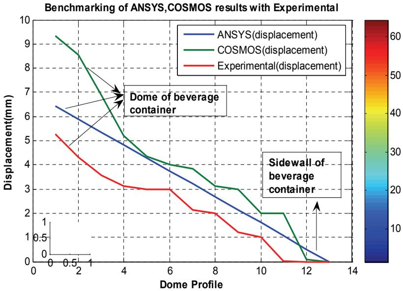
Figure 6: A comparison of displacement profile (of beverage container from sidewall to dome) obtained in ANSYS, Cosmos Works and experimental work
