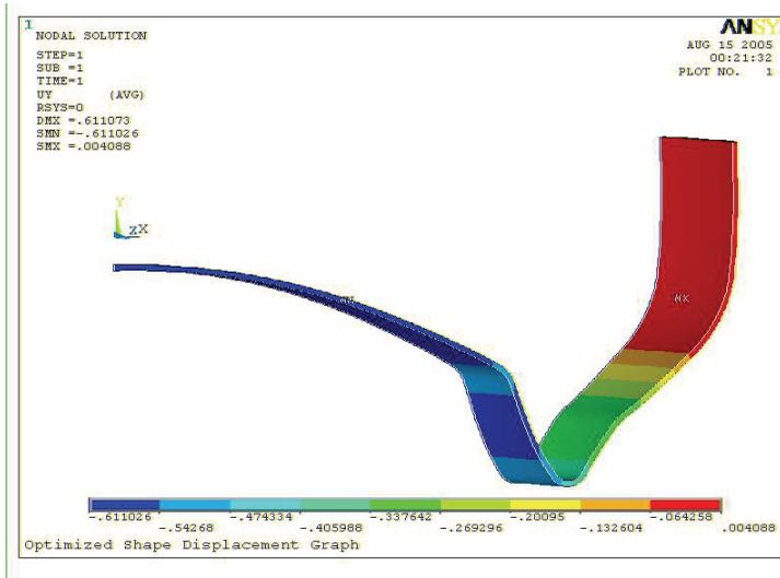
Figure 10: Optimized dome displacement graph obtained in ANSYS
