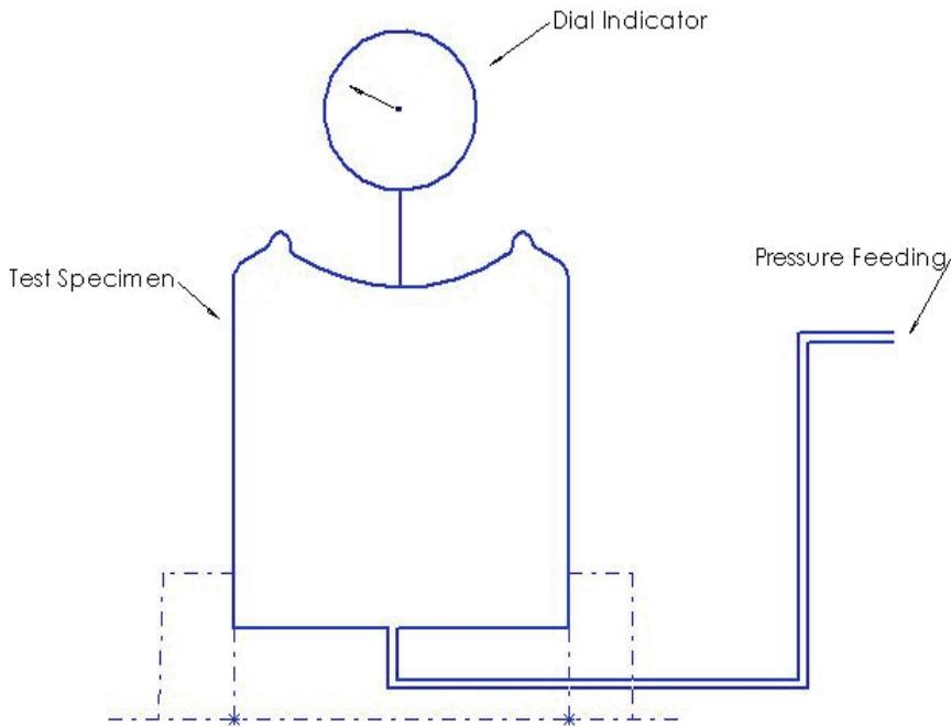
Figure 1a: Schematic of the experimental setup
