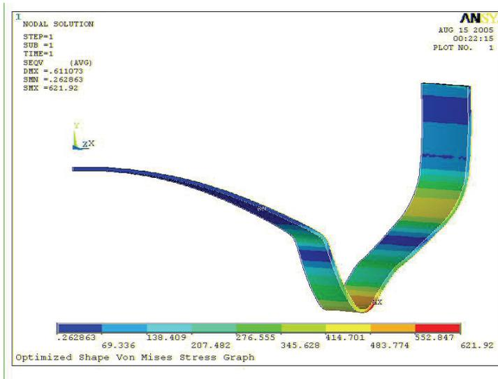
Figure 11: Optimized stress plot obtained in ANSYS using von Mises criterion
