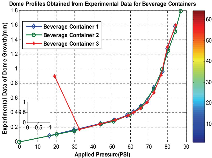
Figure 5: Dome growth profile obtained from experimental data
