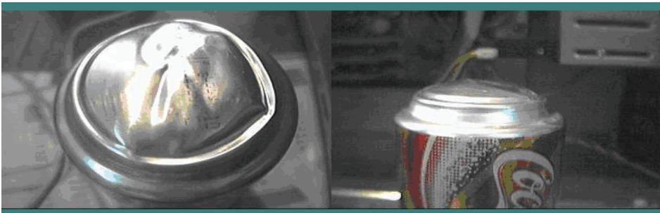
Figure 1: Dome reversal phenomenon in beverage container
