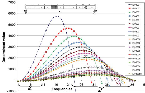
Figure 2: Variation of determinant with degree of damage (EI in  $\text{kNm}^2$ )
