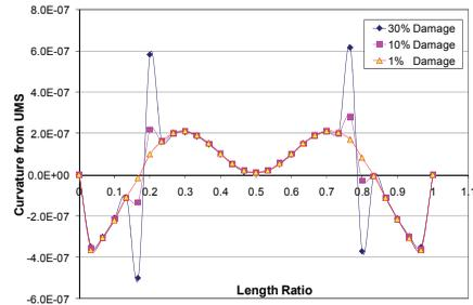
Figure 6: Curvature of Uniform Moment Surface of a beam with different damage magnitudes
