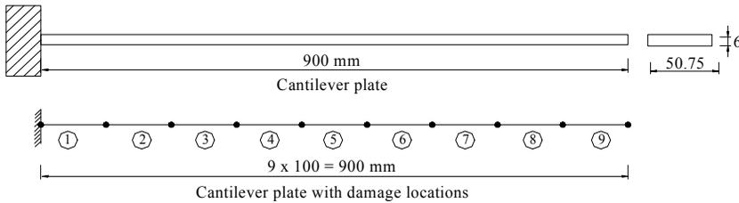
Figure 7a: Cantilever plate for simulation
