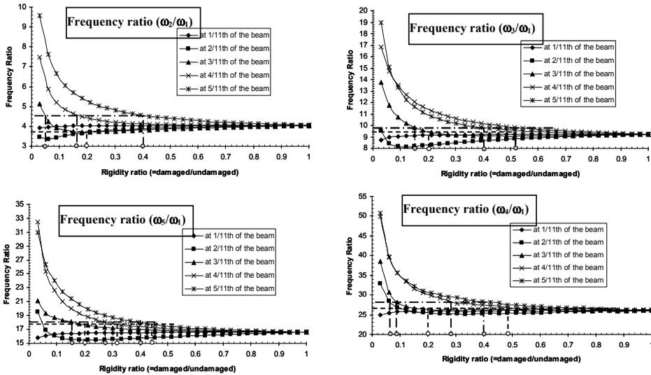
Figure 4: Identification of damage from frequency ratio
