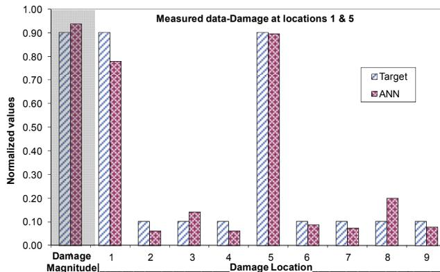
Figure 9: Damage at locations 1 & 5 for measured frequencies of cantilever beam (Target values taken from Brownjohn et al., report 2001) (6-18-10 ANN)
