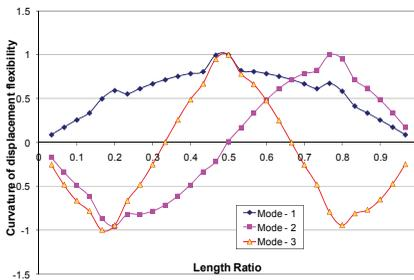
Figure 5: Curvature of modal flexibility (displacement) of a beam with damages (30%) for 3-modes
