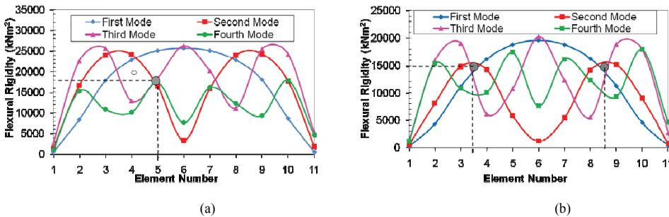
Figure 3: (a) Plot of flexural rigidity versus element diagram for a single damage case (b) Plot of flexural rigidity versus element diagram for a multiple damage case
