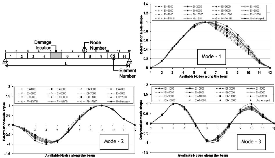
Figure 1: Difference in the mode shape of the beam for different degrees of damage in 5<sup>th</sup> element
