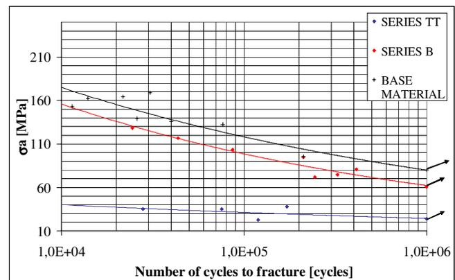
**Figure 10** : Fatigue curve of treated specimens in comparison with B and base material curves.
