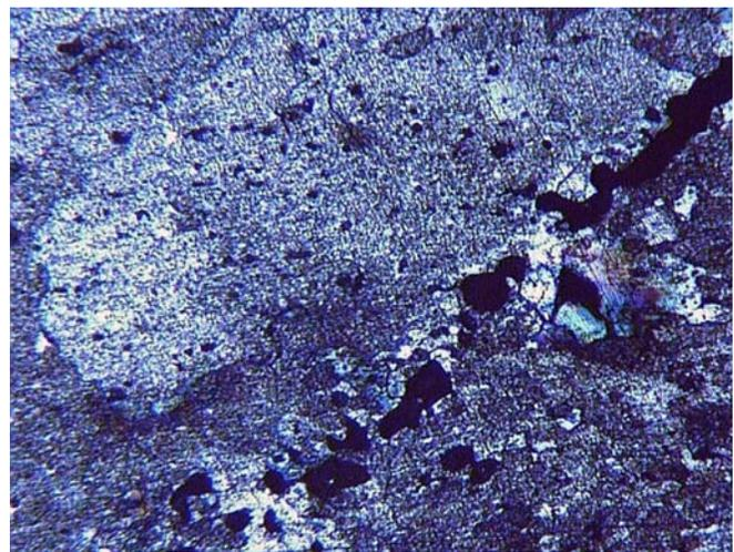
**Figure 11** : Microstructural of the grain at the interface between the nugget and TMAZ zone (125x).
