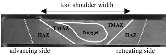
**Figure 3 :** Microstructural analysis of a FSW joint.
