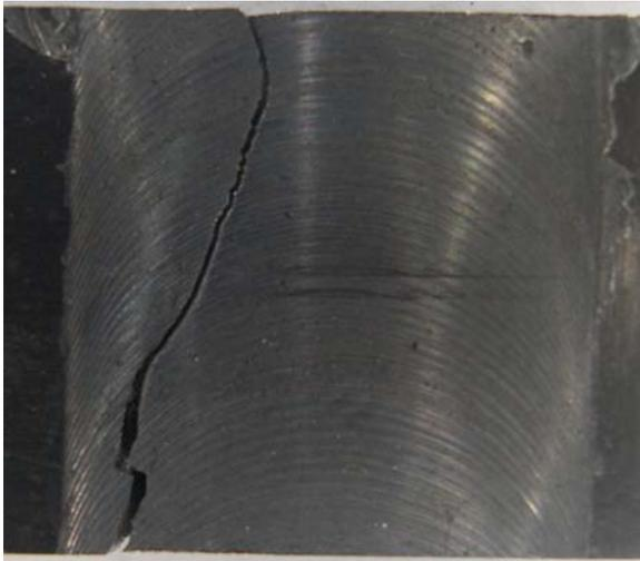
**Figure 7** : Fracture in the HAZ zone and depicting of changing of crack path.
