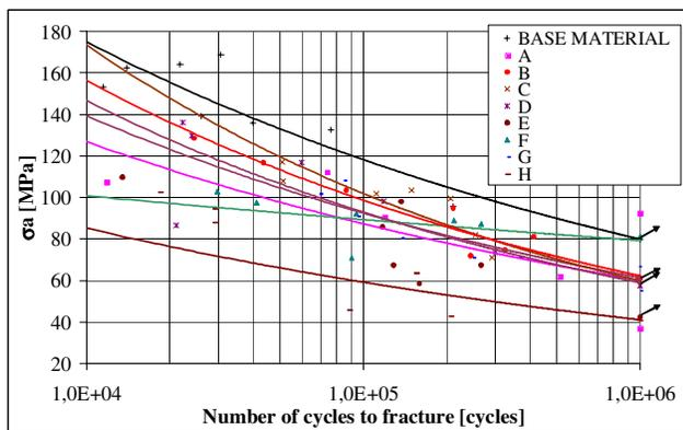
**Figure 5** : Fatigue curve of base material and FSW joints.
