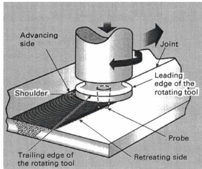
**Figure 1 :** Schematic representation of the FSW process.
