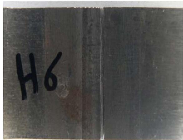
**Figure 9** : Fracture at the interface between the nugget and TMAZ zone.
