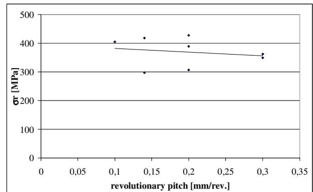
**Figure 4 :** Tensile strength as function of revolutionary pitch for each kids of joint.
