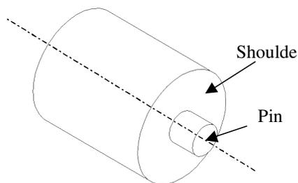
**Figure 2** : Representation of tool geometry used in the experiments.
