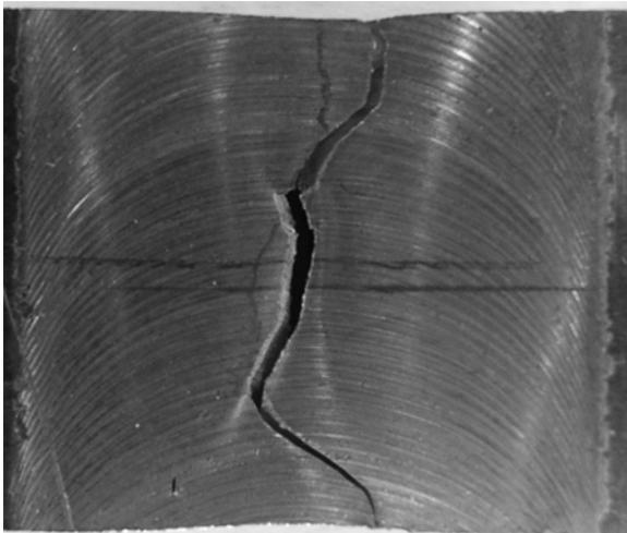
**Figure 8** : Fracture along the welding line. It shows an evident striation.
