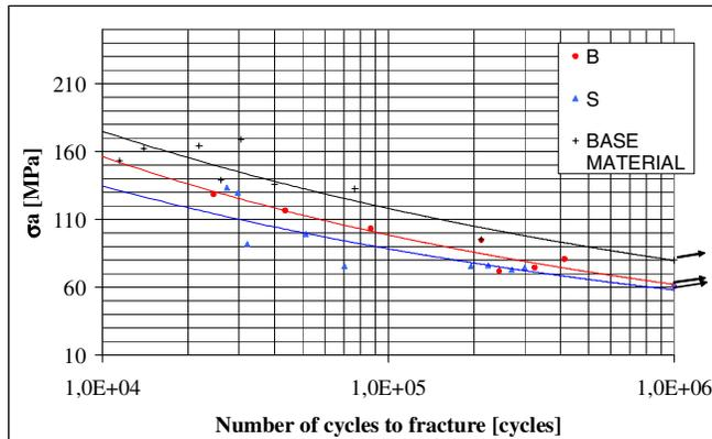
**Figure 12** : Fatigue curve of milling specimens in comparison with B and base material fatigue curves.
