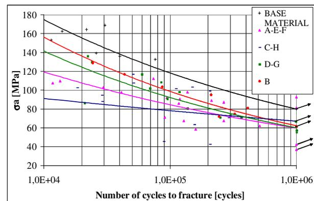
**Figure 6** : Fatigue curve as function of revolutionary pitch.
