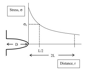
**Figure 1** : A typical notch, with depth D and root radius  $\rho$  TCD methods use the stress/distance curve: for the Point Method (PM), failure occurs when the stress at a distance L/2 is equal to the characteristic strength  $\sigma_o$ ; for the Line Method (LM), failure occurs when the average stress over a distance 2L is equal to  $\sigma_0$ .
