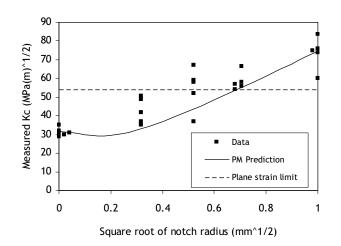
Figure 5 : Data from Tsuji et al (1999) on lowtemperature cleavage fracture of steel. Predictions using the PM (with L=0.05mm); plane strain limit value calculated using equation 7.
