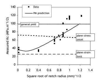
**Figure 6** : Data from Yokobori et al (1977). Predictions using the PM; estimated values for the plane strain limit, plane stress onset and general yield.
