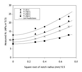
**Figure 4** : Experimental data [Srinivas and Kamat (2000)] and predictions using LM, for an aluminium alloy tested at various temperatures.
