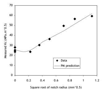
**Figure 3** : The same data as fig.2, with PM predictions using the optimum value of L (0.035mm). Results from FEA were used for the higher notch radii where they differed significantly from those of equation 4. The largest difference between data and predictions is 10.1%.
