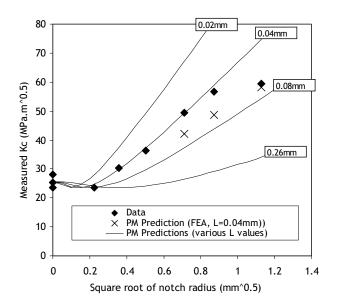
Figure 2 : Experimental data [Wilshaw et al (1968)] showing measured fracture toughness as a function of the square root of notch radius. PM predictions using stress values predicted by eqn 3 with various values of L. Further PM predictions for L=0.04mm using stress results from FEA rather than eqn 3.
