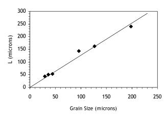
**Figure 9** : L values calculated from the data of Yokobori and Konusu (1977), plotted as a function of the grain size of the material.
