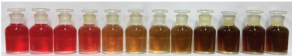
Figure 2: Color changes of KC extract at different pH levels (pH 1–12, from left to right)
