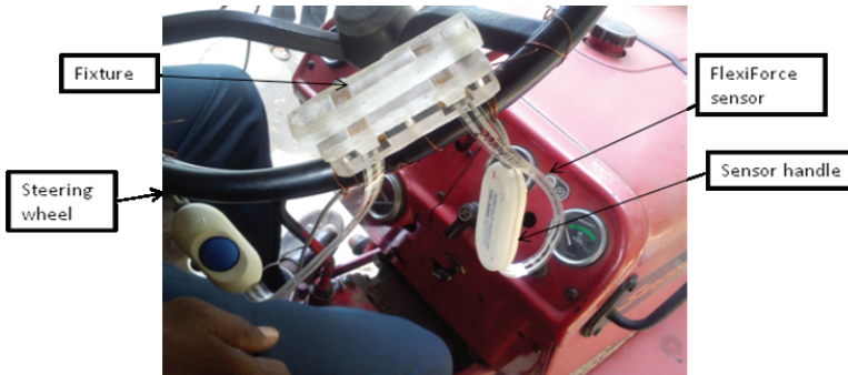
Figure 12: Fixture with sensor.
