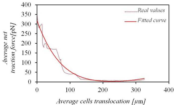
Figure 8: Average magnitude of the net traction force versus average translocation of the cells due to thermotaxis.
