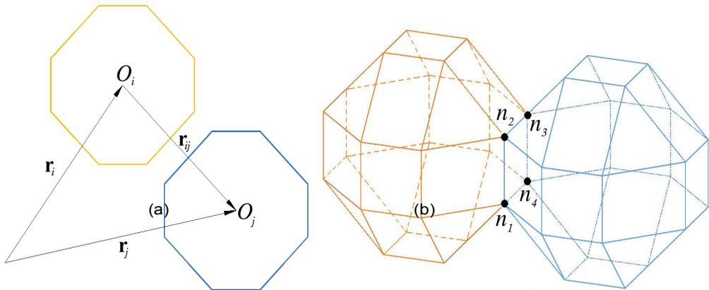
Figure 2: a. Calculation of the position vector of each cell and the distance between the centroids of two cells. The minimal distance between their centroids is equal to the proposed cell diameter. b. Interaction between two cells in contact. Here, for the assumed cell shape and discretization, two cells can have four common nodes as a maximum.
