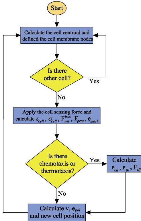
Figure 3: Computational algorithm of cell migration and cell-cell interaction considering mechanotaxis, chemotaxis, and/or thertotaxis.
