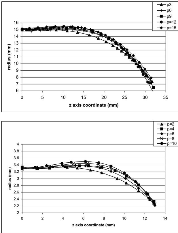
**Figure 3 :** Representation of radii obtained at pressure levels up to 15 cmH<sub>2</sub>O as function of z for one of the pig experiments (top graph) and for one of the guinea pig experiments (bottom graph). For the ease of interpretation only a limited number of the pressure levels is shown.
