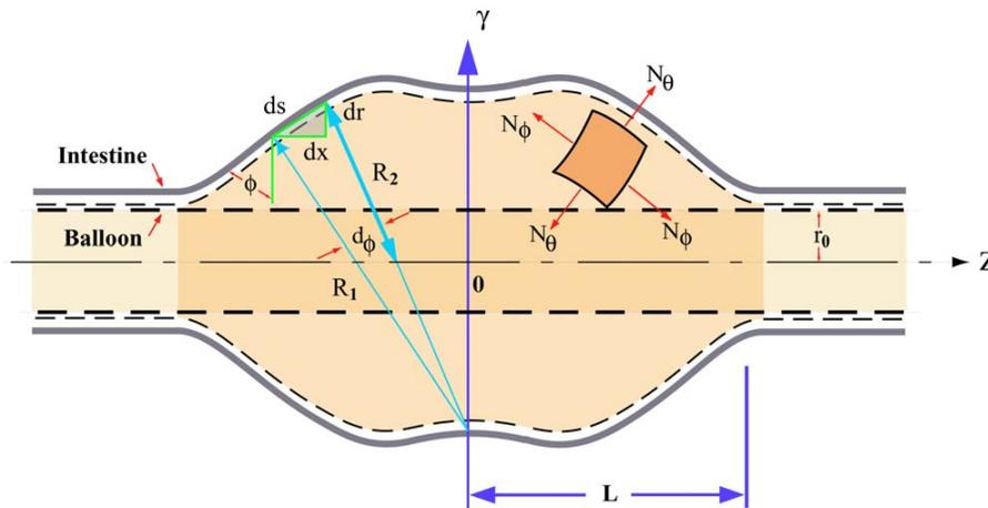
**Figure 1** : Schematic drawing of the distended segment of an intestine. Coordinates with  $z$  as the longitudinal axis,  $r$  as radial axis,  $\theta$  the polar angle,  $\phi$  the latitudinal angle.  $\theta$  and  $\phi$  form a set of curvilinear orthogonal coordinates. Membrane stress resultants are  $N_\theta, N_\phi$ , the circumferential and longitudinal membrane stress, respectively. Definitions of these coordinates and stress resultants are given in the appendix.
