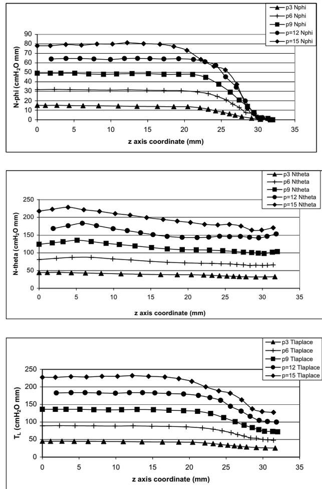
**Figure 4 :**  $N_\phi$ ,  $N_\theta$  and  $T_L$  as function of z at the same pressure levels as shown for the pig experiment in figure 3.  $N_\phi$  and  $T_L$  are seen to resemble the shape of the radii shown in figure 3 whereas  $N_\theta$  has a local maximum 20-30% away from the middle of the balloon.
