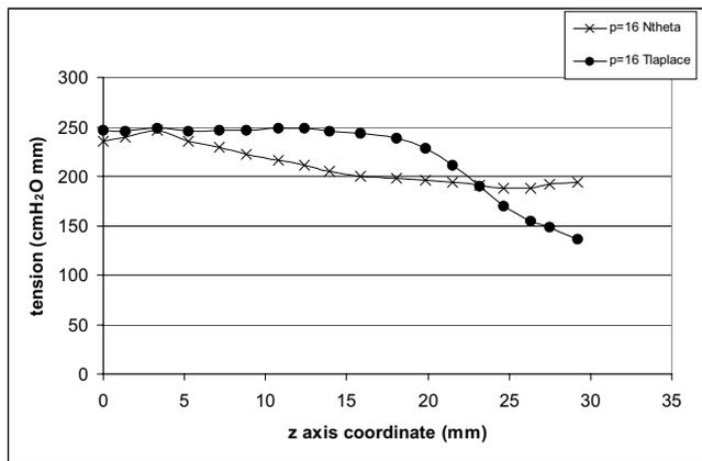
**Figure 5** : Comparison of  $T_L$  and  $N_\phi$  in a representative pig experiment at pressure 15 cmH<sub>2</sub>O. Only at the location of maximum  $N_\theta$  were  $N_\theta$  and  $T_L$  similar. At about 80% away from the middle of the balloon  $N_\theta$  became higher than  $T$ . The same pattern was found at lower pressures and using the smaller balloon in guinea pigs.
