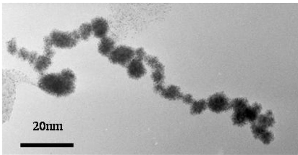
**Figure 2** : HR-TEM image of a Pt-labelled DNA fragment in the absence of MWCNTs.
