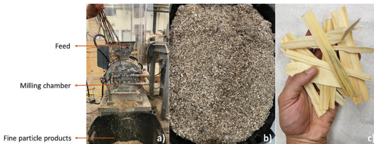
Figure 3: Preparation of cotton stalk particles for particleboard analogs: (a) hammer milling of cotton stalk; (b) cotton stalk particles after processing; (c) wood strands
