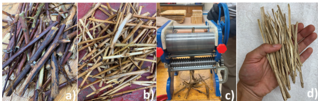
Figure 2: Processing steps: (a) wet cotton stalks; (b) bark removal; (c) converting stalks into strips using a manual noodle maker; (d) cotton stalk strips prepared for panel fabrication
