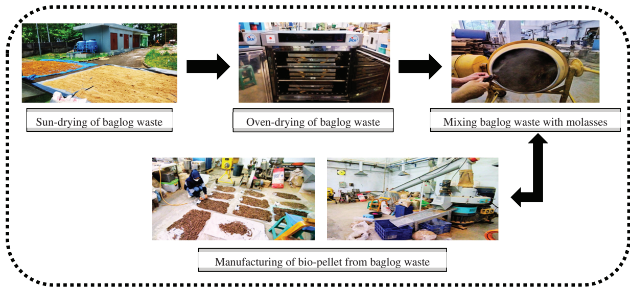
Figure 2: The schematic diagram of the bio-pellet manufacture derived from oyster mushroom baglog waste in different mixture ratios of molasses
