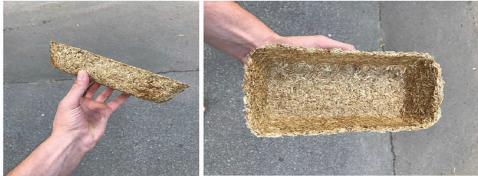
Figure 10: PBAT/PLA composites with 50 wt.% hemp stem waste tray for packaging and storing food products in the form of fruits, vegetables, and berries
